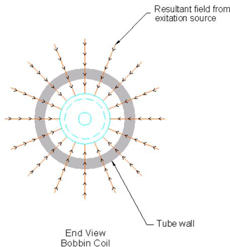
circumferential coupling between the electromagnetic field and the tube wall because the entire coil is facing the tube wall. In other words, in-line or parallel with the tube axis. The efficiency of the coupling is maximized when the coil is perfectly centered and matches the axis of the tube. As the
