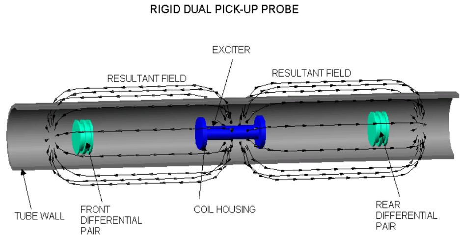
A bobbin coil is wound with magnet wire wrapped around a housing that looks similar to a seamstress's bobbin used for sewing thread. Typically, the bobbin coil centerline is positioned such that it's center is in-line with the tube axis. This creates complete
